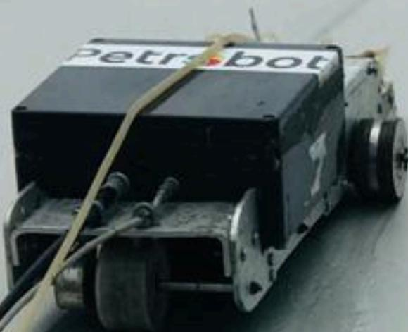
MagRover is a magnetic inspection tool that can perform non-destructive testing of assets without any scaffolding. MagRover is equipped with multiple Thickness Sensor which scans the asset faster and less riskier than Manual Inspection.
